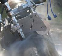
The coldcut<sup>™</sup> cobra fire extinguishing technique combines abrasive water jet cutting with water spray extinguishing.
